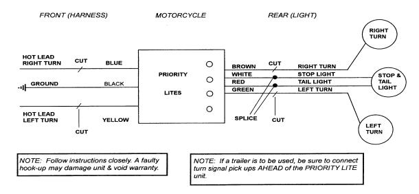
PRIORITY LITES used in conjunction with other accessories may total more amp/watt than your particular motorcycle system is capable of supporting. Please check owner's manual or local shop before installing PRIORITY LITE, or any accessory requiring power.
